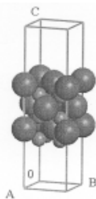
Figure 1. The view of supercell representing \text{TiH}_2 . The titanium and hydrogen atoms are represented by large and small spheres respectively. The distances are: OA = 4.528 Å, OB = 4.528 Å, OC = 27.5 Å [16]. The ratio of hydrogen and titanium atoms in this supercell is 2:1.
